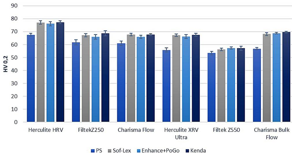
**Fig. 2.** Average values and standard deviations of surface microhardness (HV)
