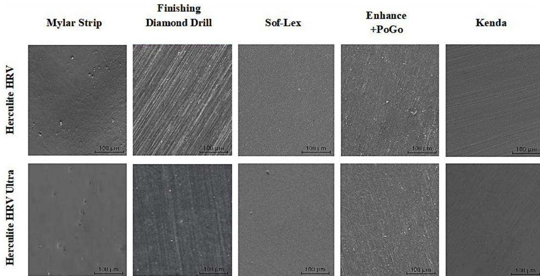
Fig. 3. SEM micrographs of the surface of control samples, finished with a diamond drill and polished using three methods on the example of Herculite HRV and HRV Ultra,  $\times 500$
