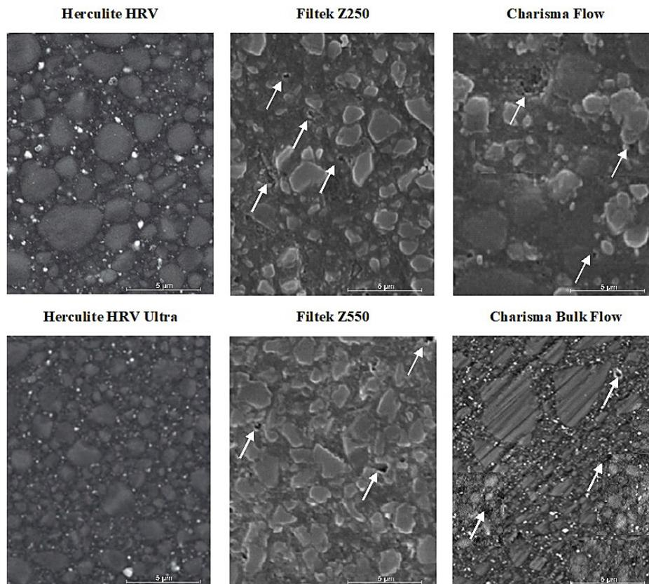
Fig. 4. Microstructure of representative composite samples,  $\times 3500$ . The arrows mark the pores revealed in the material
