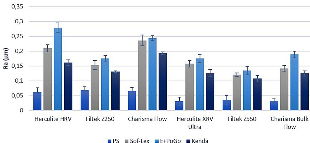
**Fig. 1.** Average values and standard deviations of surface roughness (Ra)
